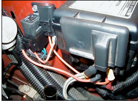
Figure 25 –Main power connection
